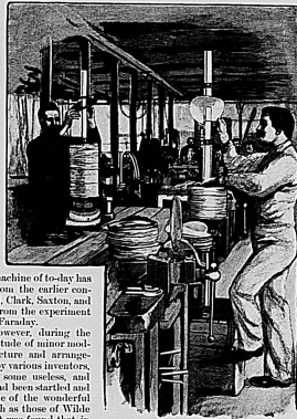
FIG. 6.—Workmen Building up the Armature Core of a Modern Dynamo.
